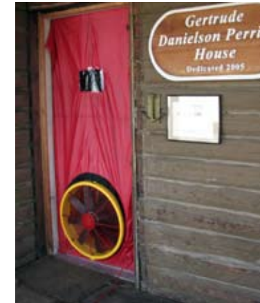
Mike Carlton's blower door on the PCEI Perrine House while measuring energy efficiency. Photo: Jen Hiebert
